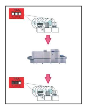
T.D.l's - An irreversible colour change from white/grey to black when standard dish washer (65°C), thermal/chemical disinfection (71°C) or thermal disinfection (82°C) temperatures have been reached.
