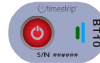
Armed and temperature breach has occurred.
