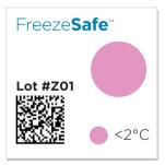
**Example:** The 2°C threshold indicator dot will be as dark as the reference dot in 90 minutes at 1°C. If exposed to 1°C for some period of time, say 60 minutes, the indicator dot will appear darker than prior to use and lighter than the reference dot.
