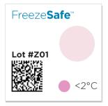
Freeze indicator activation times are based on constant temperature 1°C below the threshold. Exposure to lower temperatures will result in faster coloration and exposure to temperature above the threshold, but still within tolerance, will result in slower coloration. FreezeSafe is a cumulative color change relative to exposure time.
